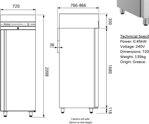
**U**INOMAK **(**) Shown on legs, supplied on castors **Technicial Specifications** Dimensions: 720 x 768 x 2115mm 830 670
