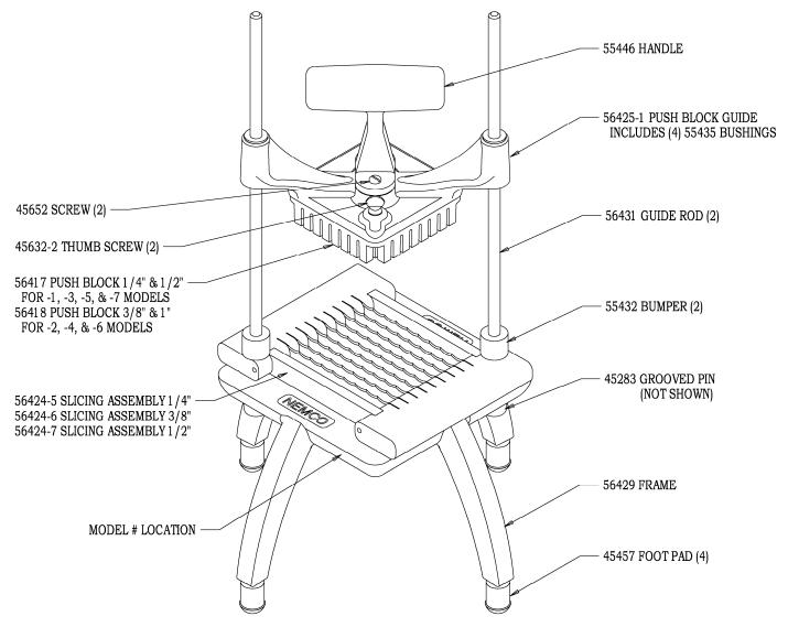
56424-1 CHOPPING BLADE ASSEMBLY 1/4" 56424-2 CHOPPING BLADE ASSEMBLY 3/8" 56424-3 CHOPPING BLADE ASSEMBLY 1/2" 56424-4 CHOPPING BLADE ASSEMBLY 1"
